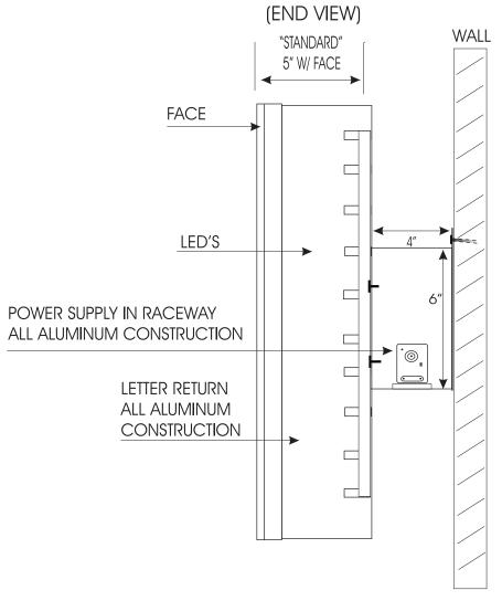
INSTALLATION: 3/8"X4' LAG BOLTS, 4 PER LETTER OR AS NEEDED (MAY REQUIRE OTHER TYPES OF FASTENERS DEPENDANT OF WALL)
